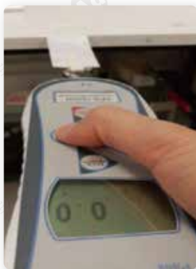
Figure 4 Ensure that the test strip and force gauge line up horizontally
